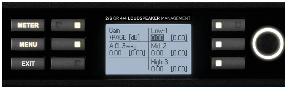
Figure 6-14: Single Module Gain Edit Screen
