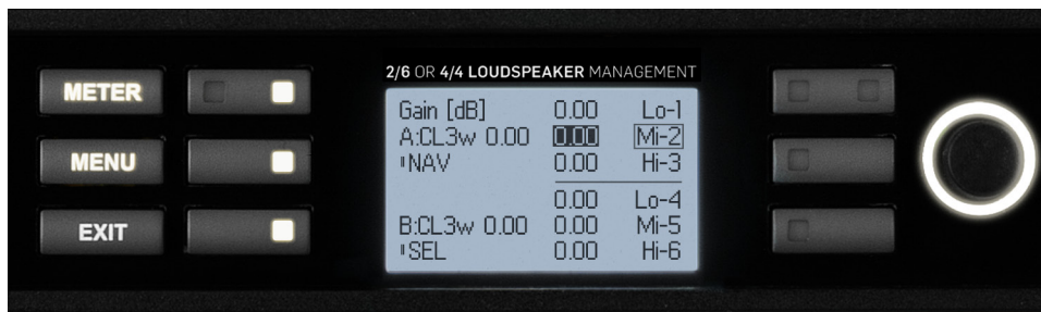
Figure 6-15: Module A+B Combined Gain Summary Edit Screen
