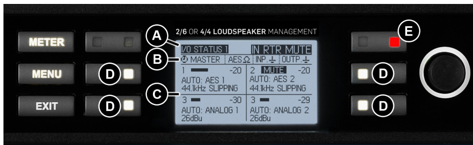
Figure 6-10: Meter Mode > I/O Status View
