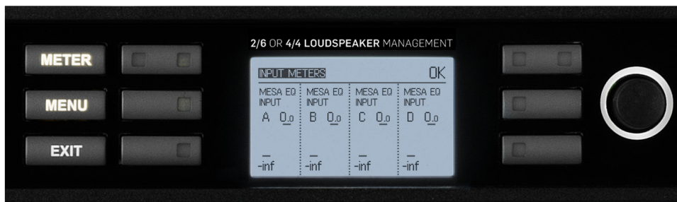
Figure 6-9: Meter Mode > Input Meters (Mesa Only)
