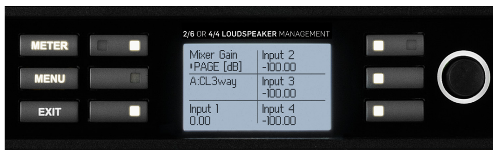
Figure 6-13: Module Input Mixer Gain Edit Screen
