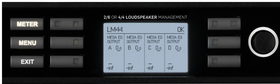
Figure 6-8: Meter Mode > Home View (Mesa - Module Outputs)
